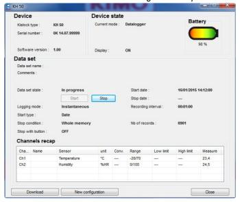
Click on "New configuration" button on the bottom left. The following window opens.
