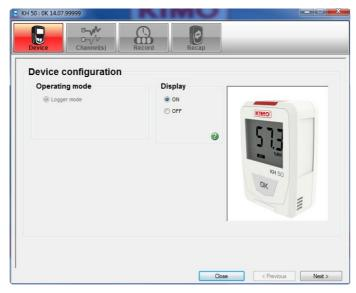
This window allows to enable or not the displaying of the values on the screen of the kistock.
