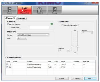
This window allows to set the channel(s) of the kistock:
